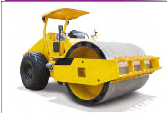
A "road roller", is a compactor type engineering vehicle used to compact soil, gravel, concrete, or asphalt in the construction of roads and foundations.
